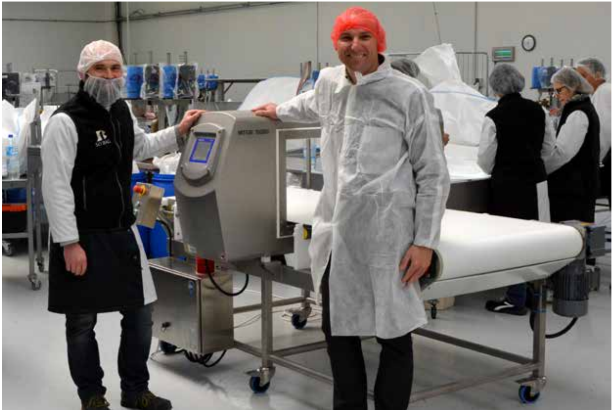
The Profile Advantage metal detection system inspecting SO BAG's FIBC bags for metal contamination.
