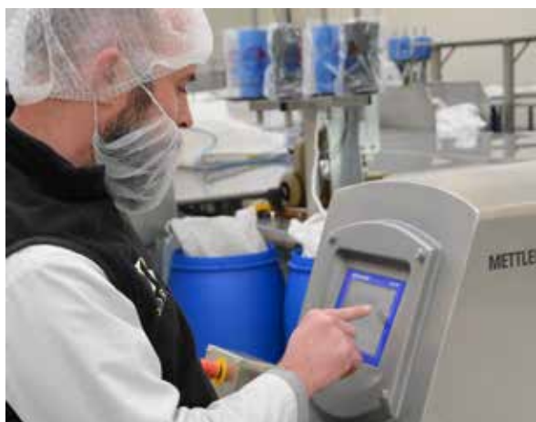
Profile Advantage technology effectively cancels out the product signal from the carbon within the bag material.
